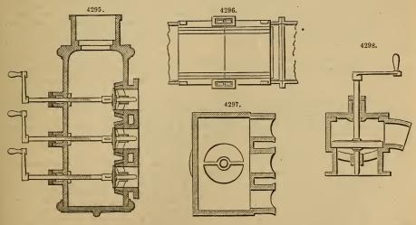
results have been obtained when the line of the blast makes an angle of 38°, and the angle enclosed by the two streams of blast 105°. Fig. 4295 is a section of a blast-valve box, with three separate valves for three tuyeres; Fig.
